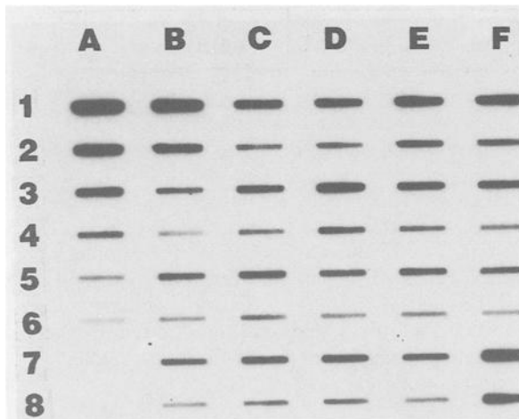
FIG. 1—An example slot blot autoradiograph derived from one laboratory's DNA extracts of 20 bloodstains. The DNA was extracted using the FBI semen stain extraction procedure and hybridized with the primate-specific probe p17H8 (locus D17Z1). Lane A contains serial dilutions of K562 quantification standards. Lanes B through F were generated using 2% (odd numbered rows) and 1% (even numbered rows) of the total DNA recovered from each stain.
